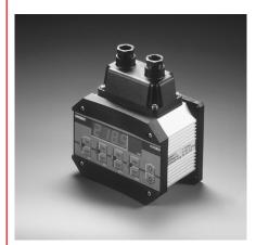
**Description:** With its integrated pressure measurement cell, 4-digit display and 4 switching outputs, the EDS 1700 offers the user all the advantages of a modern electronic pressure switch. 4 switching points and switch-back points can be adjusted very simply and independently of one another using the keypad.
