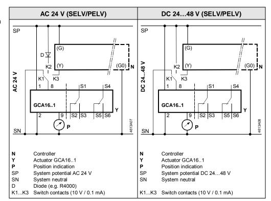
Modulating control, fully open, fully shut with GCA16..1
