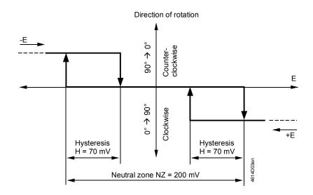
The diagram shows the relationship between the differential voltage E = Y - U (difference between setpoint Y and actual value U) and the direction of rotation, including hysteresis and neutral zone.
