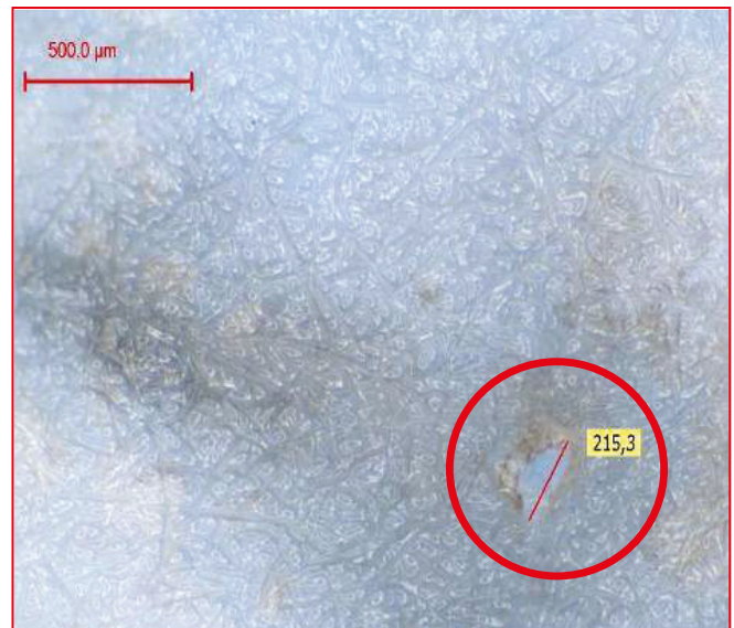
Burn hole in the filter material
