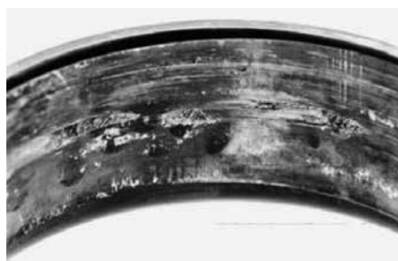
Adhesion on ball bearing
