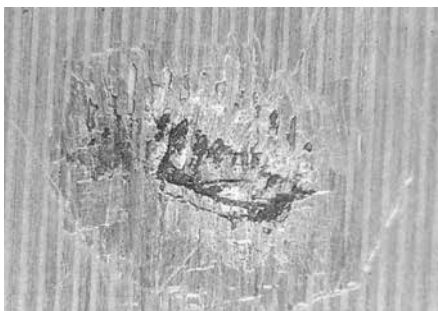
Surface fatigue on ball bearing
