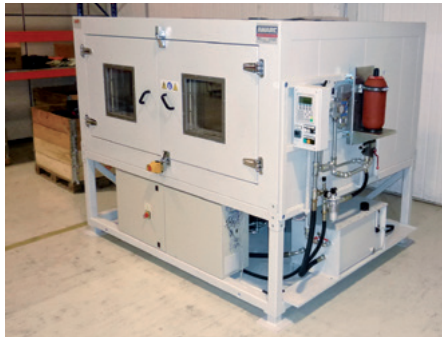
Pressure pulsation test rigs
