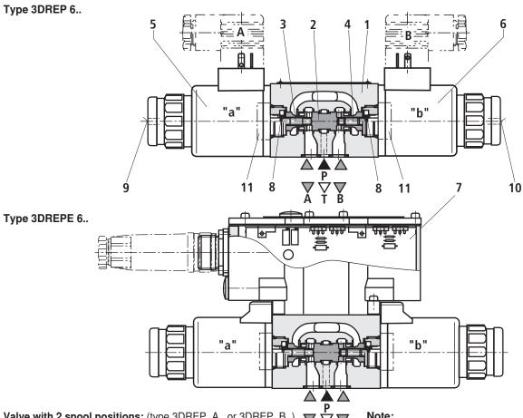
Valve with 2 spool positions: (type 3DREP..A.. or 3DREP..B..) The function of this valve design corresponds basically to the valve with 3 spool positions. The 2 spool position valves are, however, only equipped with solenoid "a" (5) or solenoid "b" (6). Instead of the 2nd proportional solenoid, there is a plug screw (11).
